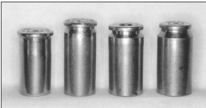
Left to right: Rimmed, semi-rimmed, rimless, and rebated rim
